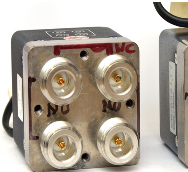
Figure 12- Coax changeover relay
