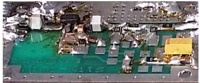
Figure 3 LNA showing output Attenuator
