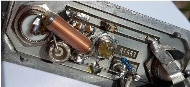
Figure 10- Reworked Commercial Bias Tee
